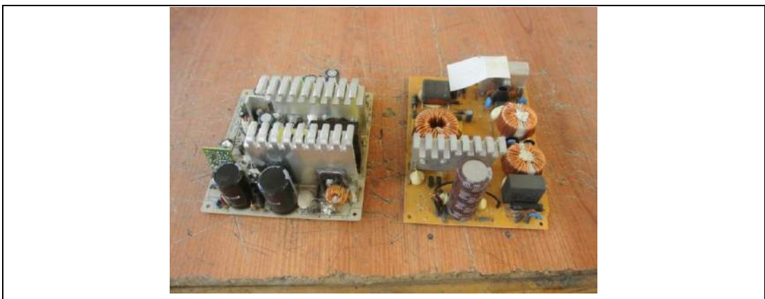
Figure 6: Internal power supply units from electrical or electronic appliances
