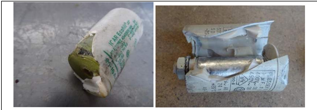
Figure 21: Opened plastic capacitors without liquid substances
