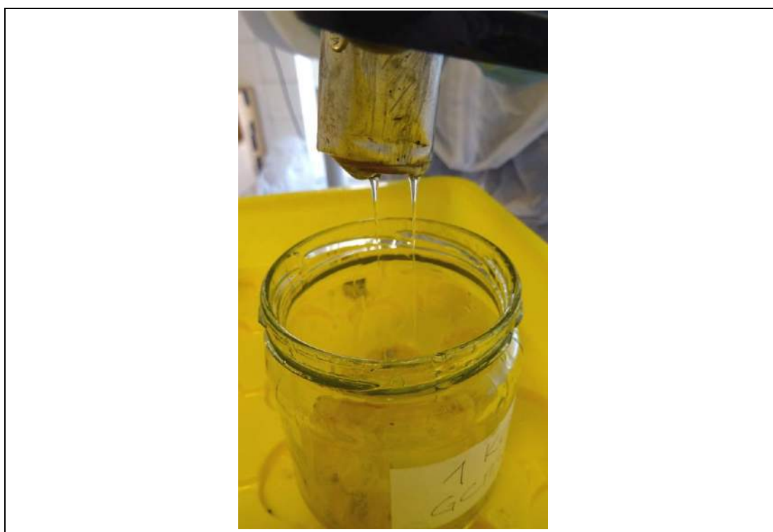
Figure 11: Liquid flowing from a non-polarised cylindrical capacitor after cutting
