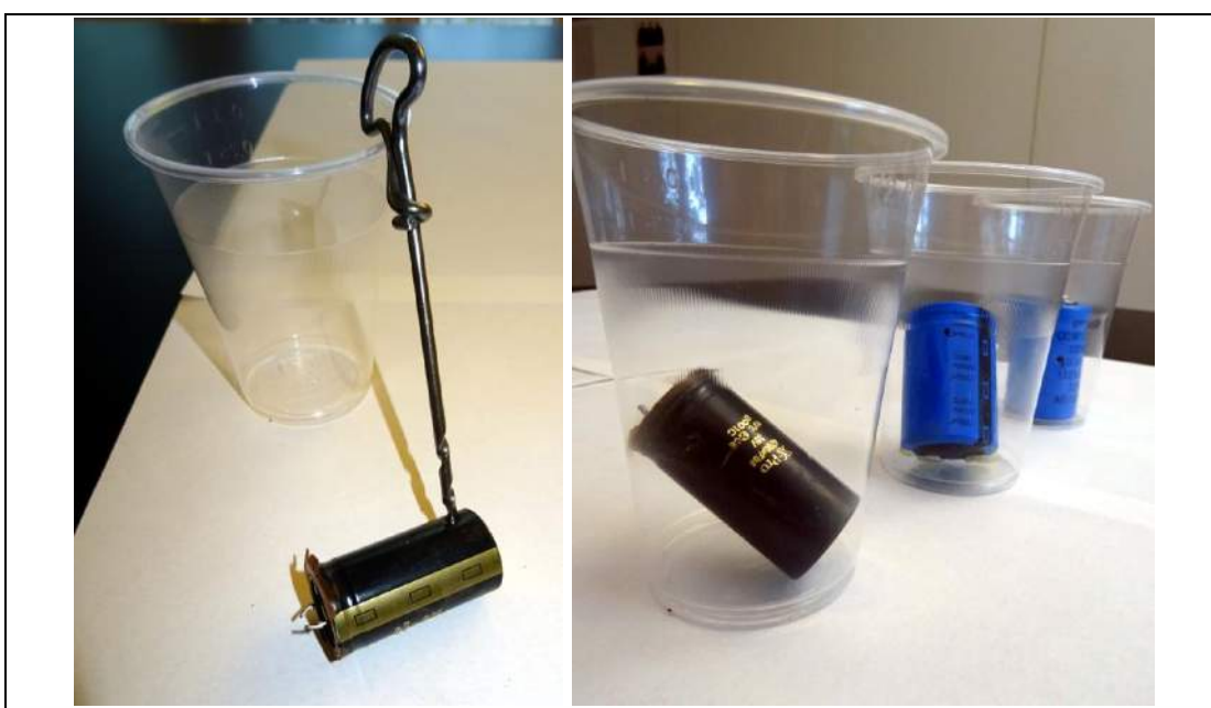
Figure 12: Piercing the e-caps and dry containers after a 13-day test period
