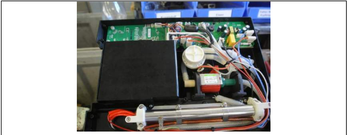
Figure 9: Interior of a steam iron station
