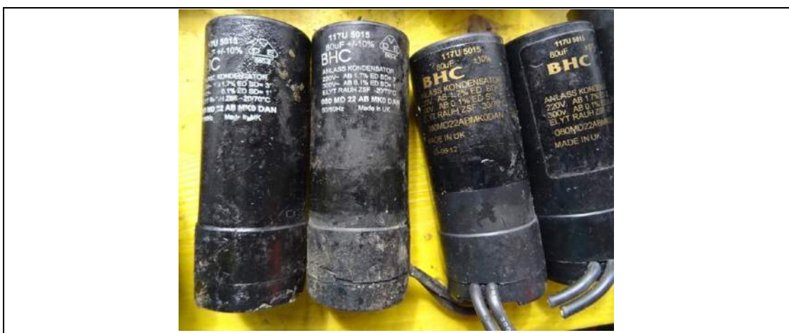
Figure 22: Motor start electrolytic capacitors in black plastic housings
